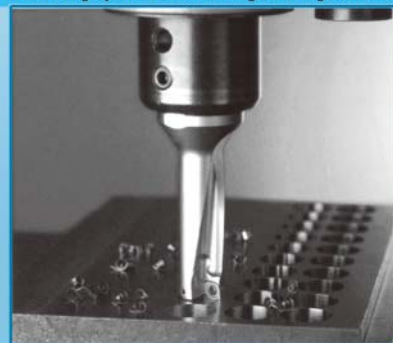
各式新型快速鑽、深孔鑽、大孔徑鑽頭 Indexable drills, deep and big hole drills
